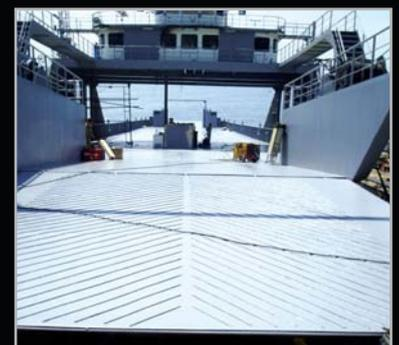
Epoxy Zinc Phosphate Primer + Epoxy Base + Epoxy Top Coat
